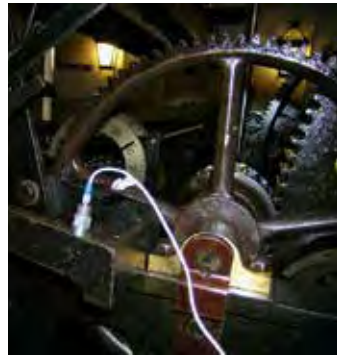
Accelerometer on the clockwork of Big Ben
