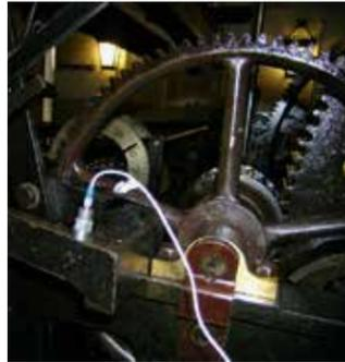
Accelerometer on the clockwork of Big Ben
